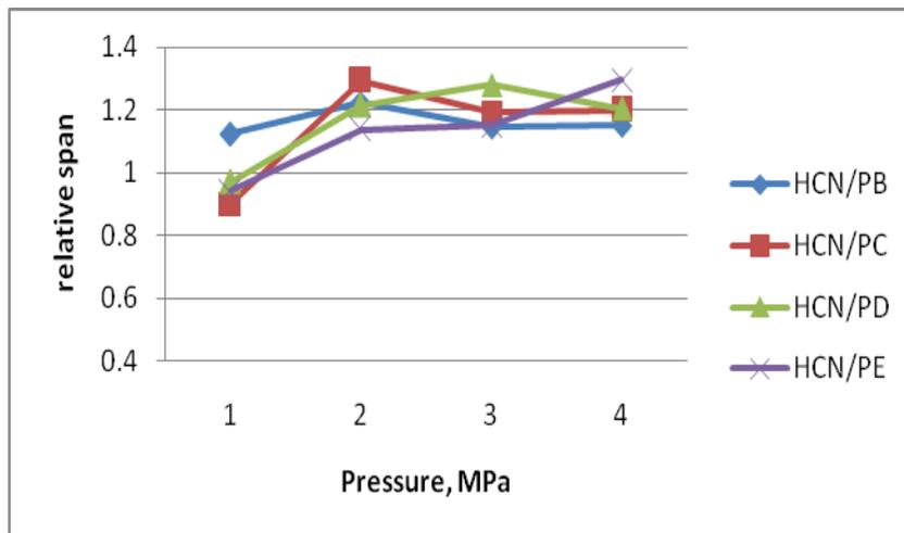
**Fig.4** Droplet size distribution of HCN/PB, HCN/PC, HCN/PD and HCN/PE nozzles at varying pressures
