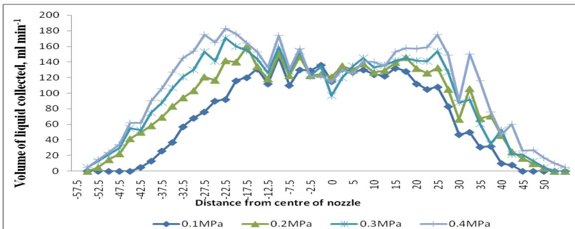
**Fig.6d** Spray distribution of HCN / PE at different pressure
