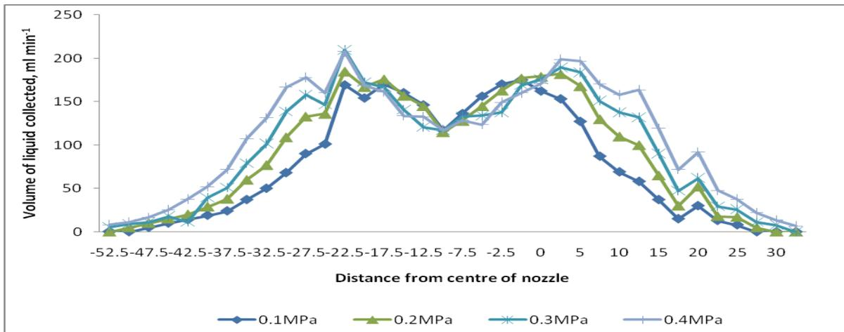
Fig.6c Spray distribution of HCN / PD at different pressure
