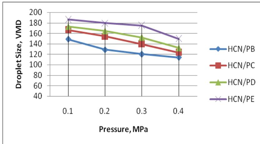
Fig.3 Effect of pressure on relative span of droplets from various nozzles
