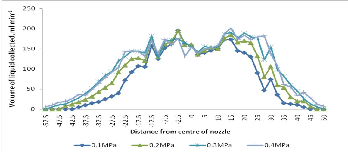
**Effect of pressure on spray angle and spray width**
