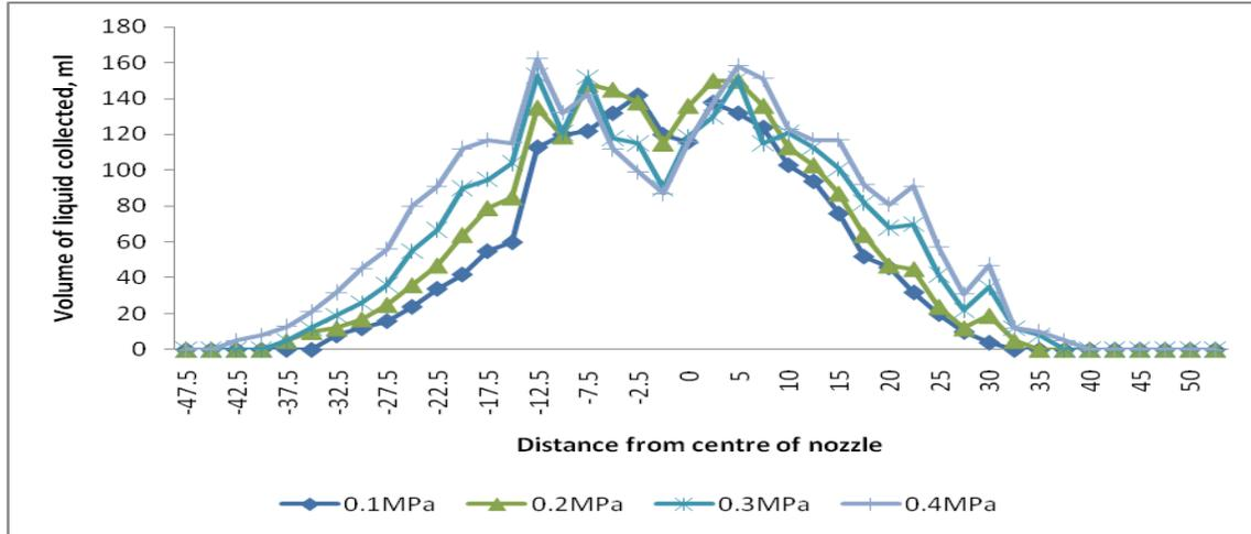
Fig.6b Spray distribution of HCN / PC at different pressure
